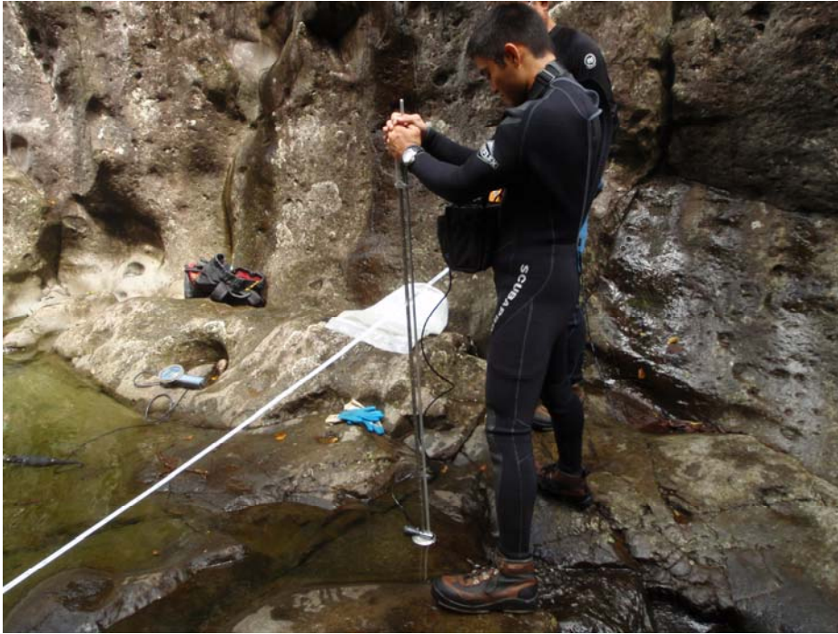
Figure 5-20. DAR staff taking flow measurement on Honomanū Stream below survey site 1. (6/28/2009; Tributary name: Honomanū (64009003); PBN: sh001p-055-062809; Surveyor: Hau, S.; SBN: 122; Lat. (DD): 20.84272, Long. (DD): -156.17705).
